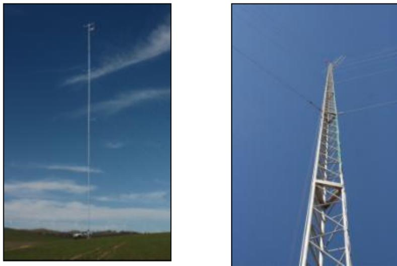
**Image 4: Tubular (left) and lattice (right) wind monitoring masts**
