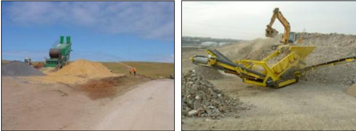
**Image 9: Temporary on-site concrete batching plant and rock crusher**
