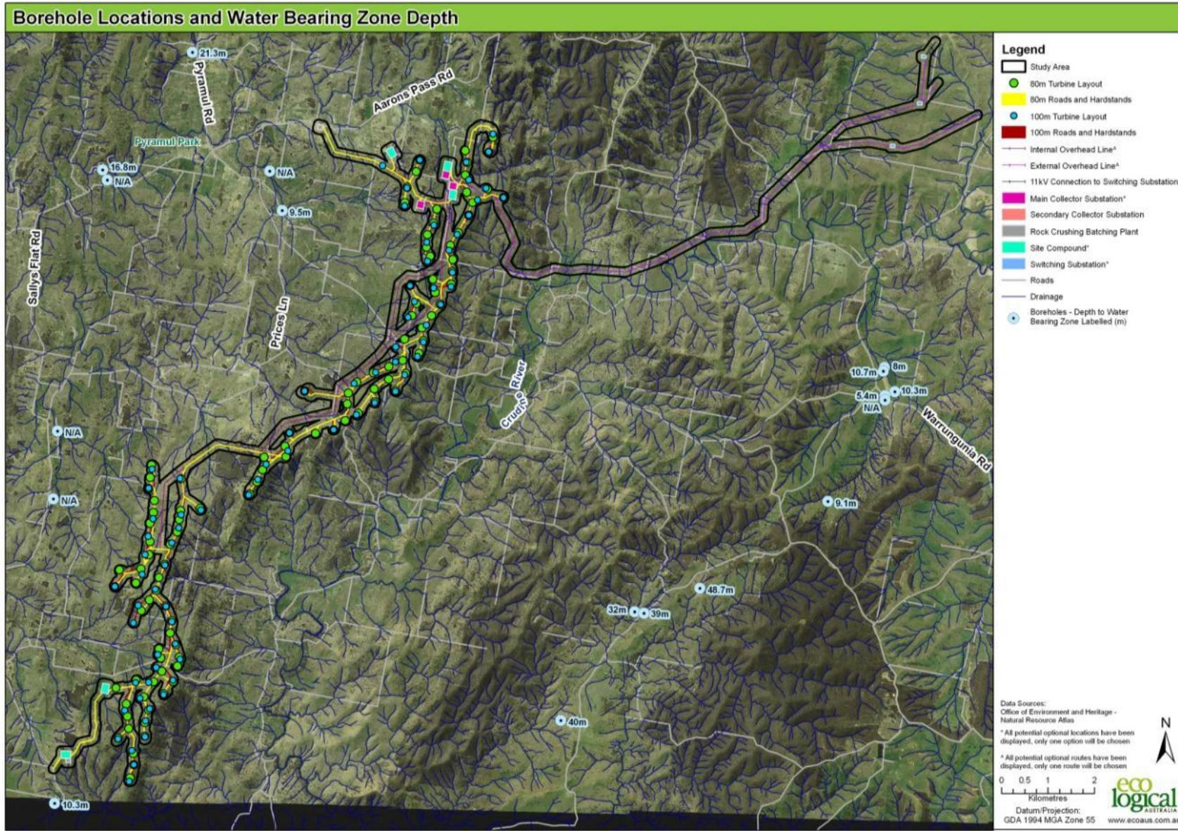
Figure 11: Groundwater bores (and water bearing zone depth) within a 10 km radius of the Project
